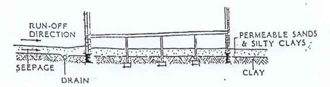
Where this occurs it is recommended that an agricultural drain be installed to divert the flow of water around the house site. Any such drain should penetrate the impermeable clay by approximately 200mm
