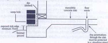
Because most concrete slabs have some penetrations through them, these must be protected by using one of the other approved materials or methods of management. Particular attention should be given to any penetrations or control joints, since access to these areas is extremely difficult later.
